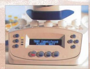
tray (Pocket) or with a 10 position fixed tray (Pocket) or with a 110 position rotating tray for 2 ml or 2.5 ml vials (Daisy Wheel). Syringes of 1 to 100ul may be used with the option of a special large injection version of up to 10 ml per sample.
